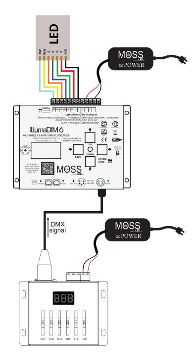
Note: The Six channel fader dimmer can output 6 channels of DMX to any receiver, it does not require an IllumaDIM 6.
