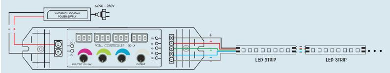
**2: Wiring Diagram for using Power Amplifier** (4 channel rotary controller dimmer can share the same power supply with the power amplifier)
