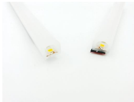
4 - It is now separated in two strips. The soldering pad is available at both strips, you can block one strip with the end caps and solder the lead wire to another strip, please follow step 5-->
