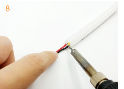
8 - Solder the wire on the strip.
