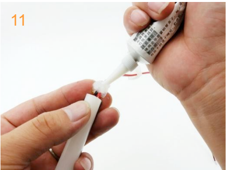
11 - Put glue on the inner end caps.
