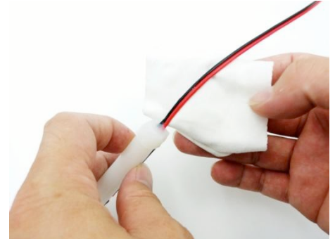
14 - Clean the glue vestige on the wire.
