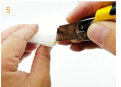
5 - Using the knife, carefully remove the silicone on the soldering pads.
