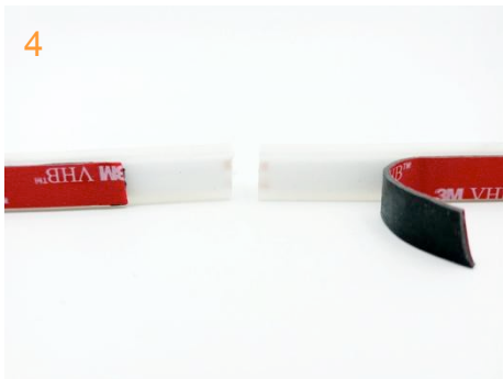
4 - It is now separated in two strips. The soldering pad is available at both strips, you can block one strip with the end caps and solder the lead wire to another strip, please follow step 5-->
