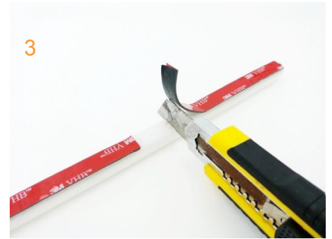
3 - Use the knife or scissors to cut off the strip at the middle of the cut
