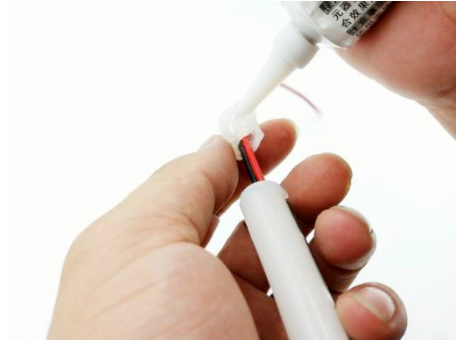
13 - Put glue on the inner end caps.
